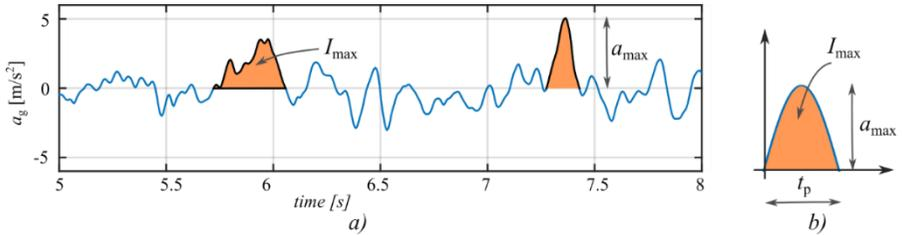
**Fig. 28** An acceleration record and the definition of  $a_{\max}$  and  $I_{\max}$ , (a), and the replacement sine curve (b). The record is the 1979, Imperial Valley – Bonds Corner/140 (NF-3)
