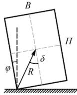
**Fig. 4** Geometry of the rigid block (the aspect ratio is:  $H/B=\cot\delta$ , moment of inertia about the corner point is  $\theta = \frac{4}{3}R^2m$ , where  $m$  is the total mass)
