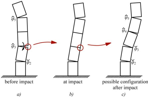
**Fig. 14** Configuration before (a), during (b) and after (c) the impact
