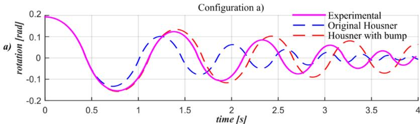
**Fig. 10** Example of the experimental results for configuration a) investigating the block with slenderness 3.7
