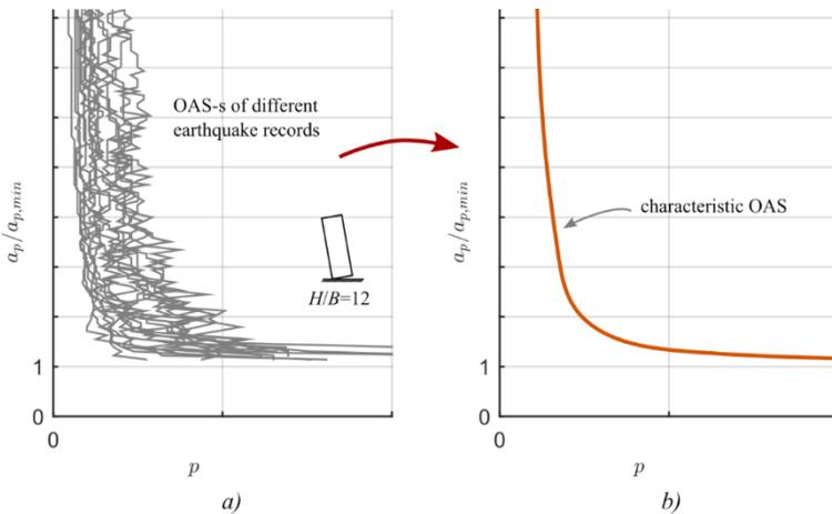
**Fig. 26** OAS-s at a given location (a) and the determined *characteristic OAS* (b)
