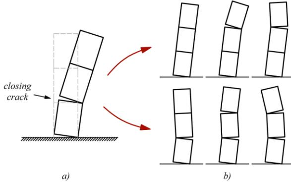
**Fig. 15** The possible rocking motions after impact ( $n^{\text{closed}}=1$ )
