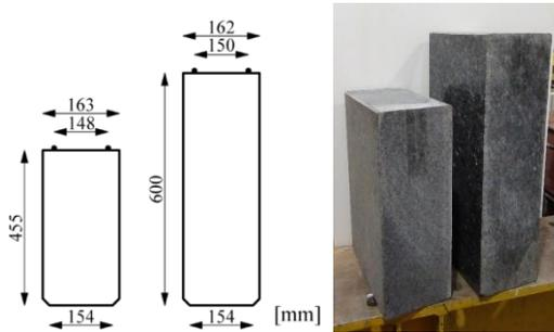
**Fig. 8** Picture and the sizes of granite blocks used in the experiments
