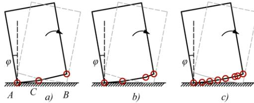
**Fig. 6** Rocking block. one bump in the middle (a), two bumps (b), several bumps (c)
