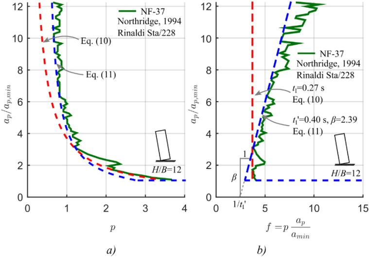
**Fig. 27** OAS (a) and transformed OAS (b) for the Northridge earthquake compared to simplified curves ( $t=0.27$ ,  $t'=0.40$ ,  $\beta=2.39$ )
