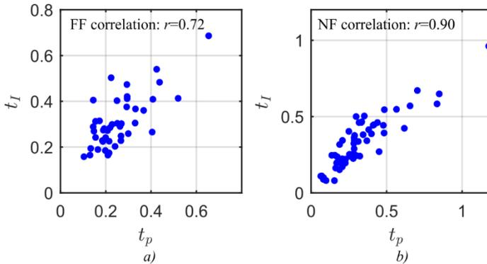
**Fig. 29** The corresponding  $t_I$  and  $t_p$  values for the FF (a) and the NF (b) records. The correlation coefficients are 0.72 and 0.90 for FF and NF, respectively
