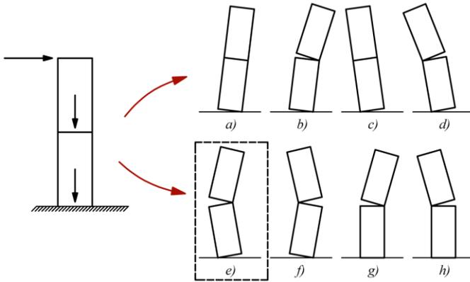
**Fig. 16** Possible openings of a two-block column
