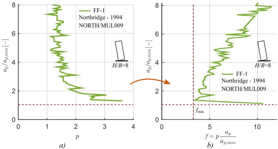
**Fig. 23** The OAS (a) and the transformed OAS (b) for an earthquake record (Northridge – 1994, North/MUL009 component)
