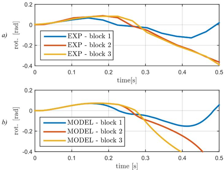
**Fig. 20** The experimental (a) and numerical (b) results of a base excitation test
