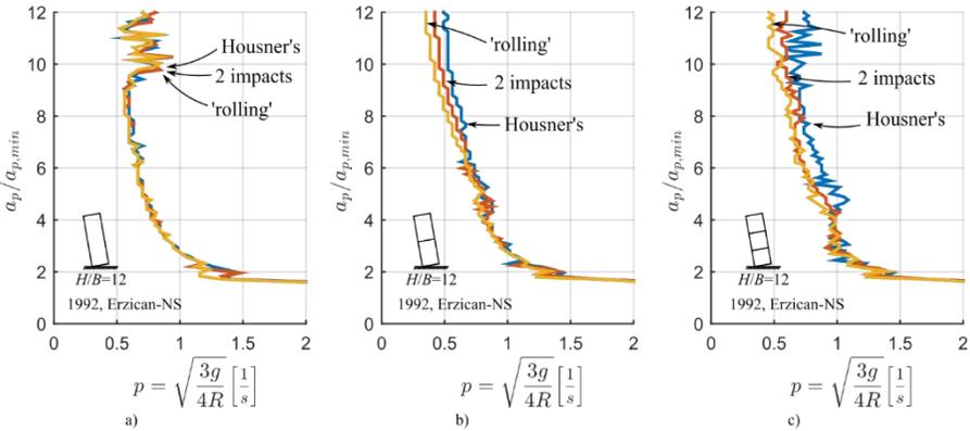
**Fig. 25** The OAS of columns consisting of 1, 2 and 3 blocks with different energy dissipations. The column is subjected to 1992, Erzican-NS earthquake record.
