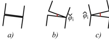
**Fig. 12** Opening possibilities of an interface (closed (a), open clockwise (b) and counterclockwise (c))
