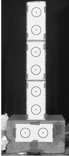
**Fig. 19** The three-block column made of granite blocks
