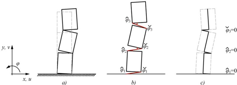
**Fig. 13** The degree of freedom of the model. One possible shape of a three-block system (a), the theoretically possible motions (b) and the choice of the zero and non-zero rotations (c)
