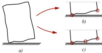
**Fig. 7** Comparison of Housner’s model and the modification with an additional bump in the middle
