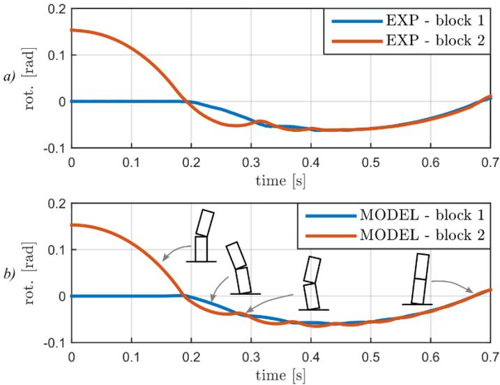
**Fig. 18** The recorded (a) and the simulated (b) rotations of the two-block system during the free-rocking experiments
