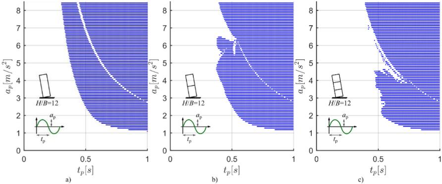
**Fig. 24** The overturning of columns ( $H=12$  m,  $B=1$  m) consisting of 1, 2 and 3 blocks subjected to full sine pulse. The dots represent overturning.
