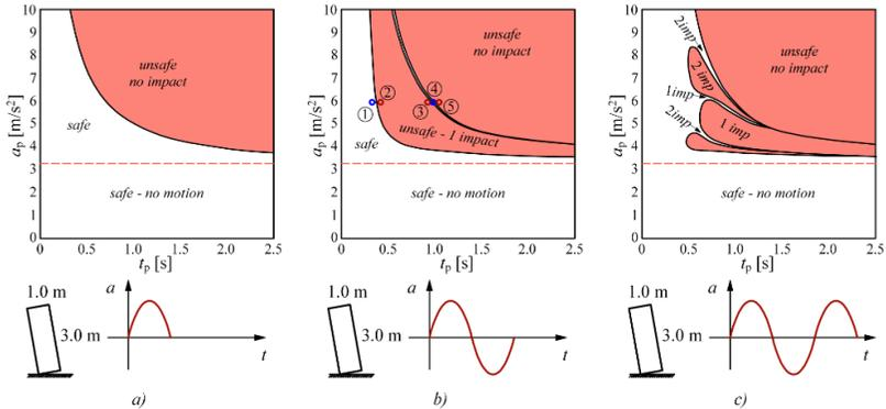
**Fig. 5** Overturning curve (OC) for a single block subjected to a half sine pulse (a) a full sine signal (b) and for a signal of three half sines (c)
