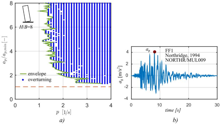
**Fig. 22** The *Overturning Acceleration Spectrum* (OAS) of a single block (dot represents overturning) (a) based on the Northridge-1994, NORTHR/MUL009 record (b)
