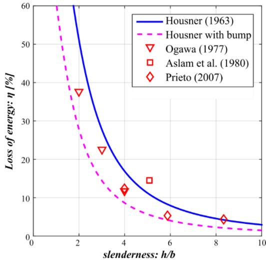
**Fig. 11** Experimental results compared with the classical Housner’s model and with the refined model including a bump in the middle.
