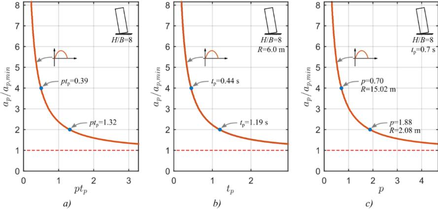
**Fig. 21** Normalized overturning curve (OC) for a single block subjected to a half sine pulse (a) (see Housner (1963)). The OC shows the effect of the pulse length (b) while the OAS shows the effect of the block size (c).
