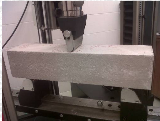
Fig. 3 – Position of the load and supports of the beam specimen.
